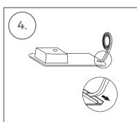
FIT GASKET TO SINK ENSURING DOUBLE THICKNESS AT THE CORNERS AND/OR USE SILICONE SEALANT TO ENSURE A GOOD SEAL
