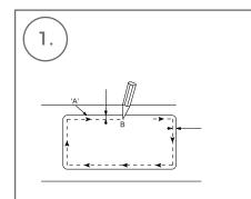
USING THE CUT OUT TEMPLATE PROVIDED, MARK THE CUT OUT LINE ON THE BENCHTOP
