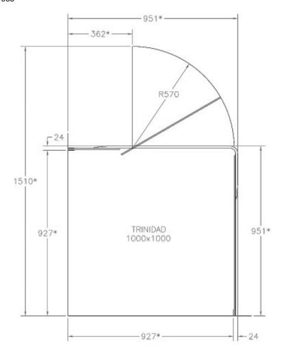
\*Note that this dimension may be increased by up to 16mm by pulling the glass further out of the wall channel.
