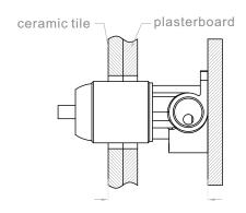
4. Remove the plastic sleeve, grub screw and water testing plug.
