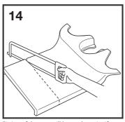
Fitting of the seat will be made easier if a sharp knife is used to put a bevel on the cut
