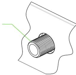
1. Apply thread sealant or teflon tape on outlet thread.
