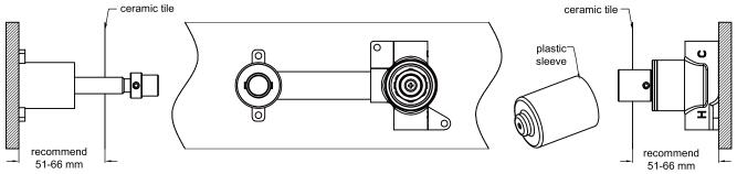
2. Connect cold water hose and hot water hose, take off plastic sleeve and conduct water pressure test for leak.
