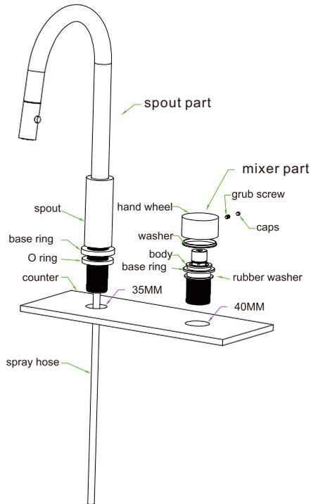
1. Drill a 35mm (for spout) and a 40mm (for mixer) through-hole on the counter. (The counter thickness must be between 20mm to 40mm)
