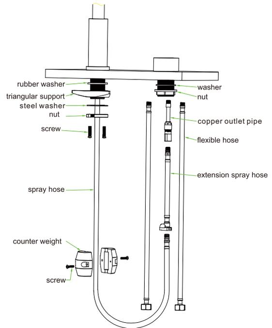
3. Slide rubber washer, triangle plate and steel washer and lock nut onto spout part in a row according above diagram. Then slide rubber washer and nut onto mixer part.
