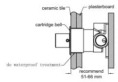
6 .Put cartridge bell onto body and do waterproof treatment.
