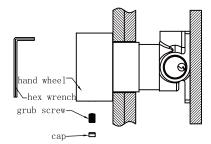
7. Make hand wheel cover on connecting rod, tighten grub screw of hand wheel by hex wrench, put cap into hand wheel.
