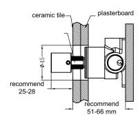
3.Adjust connecting rod and ensure depth is 25-28mm from the front of adaptor to ceramic tile.
