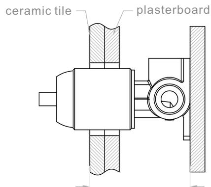
4. Remove the plastic sleeve of body.
