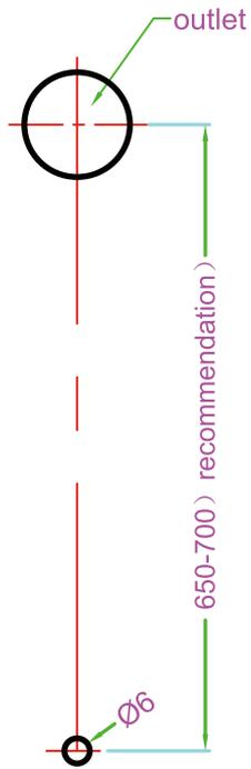
1. Drill a  $\phi 6$ mm hole at the outlet vertical downward position in the recommended range.
