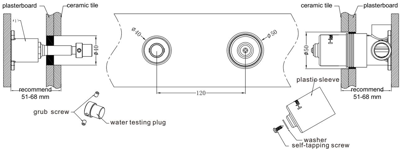
1. Install ceramic tile after drilling a  $\phi 50$  and a  $\phi 40$  hole according to above picture.
