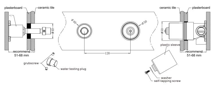
1.Install ceramic tile after drilling a  $\phi50$  and a  $\phi40$  hole according to above picture.
