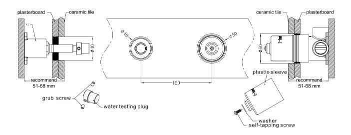
1.Install ceramic tile after drilling a  $\phi 50$  and a  $\phi 40$  hole according to above picture.
