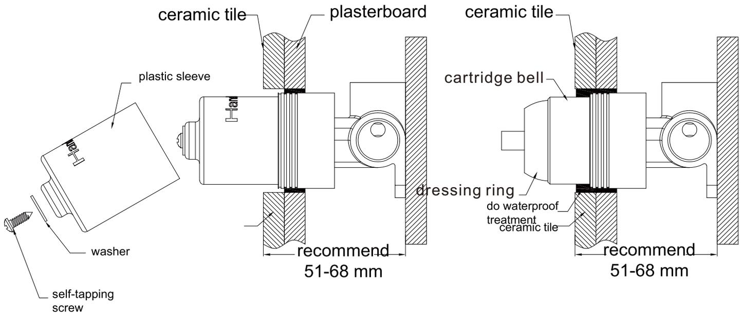
1. Install ceramic tile after drilling a  $\phi 50$  and a  $\phi 40$  hole according to above picture.
