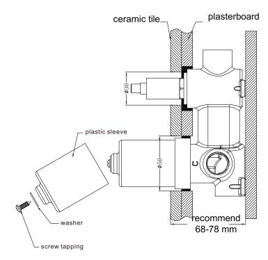
1.Install ceramic tile after drilling a  $\varphi$ 50 and a  $\varphi$ 30 hole according to above picture. 2.Take off self-tapping screw, washer, plastic sleeve.
