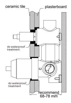
3.Put on cartridge bell and sleeve .4.Screw on dressing ring.5.Do waterproof treatment for gap
