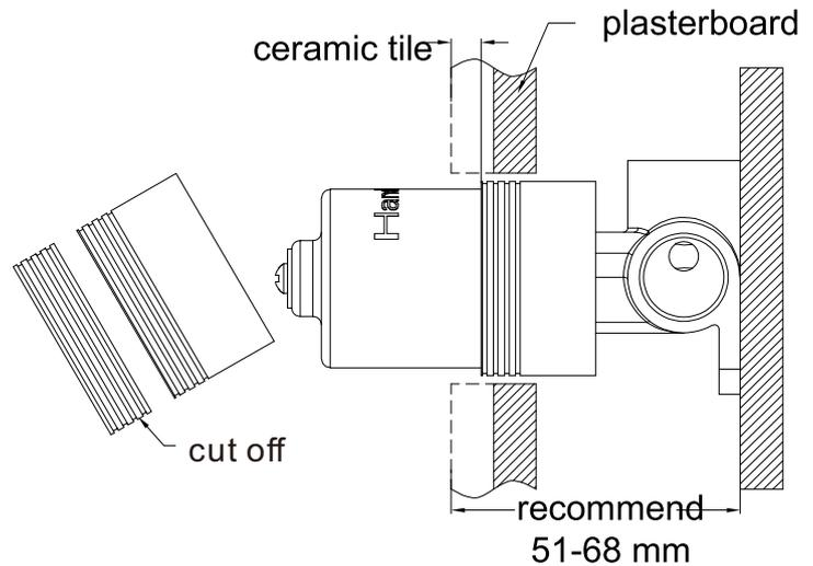
1. Fix body (1) on noggin and ensure installation depth is 51-68mm from noggin to ceramic tile.
