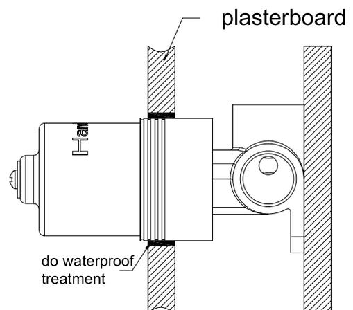
7. Do waterproof treatment for gap of plasterboard and body.
