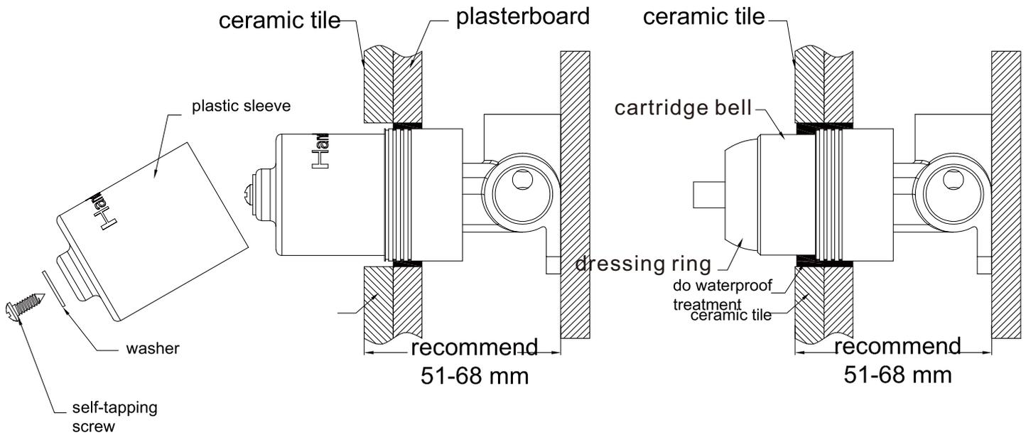
1. Install ceramic tile after drilling a  $\phi 50$  hole according to above picture.
