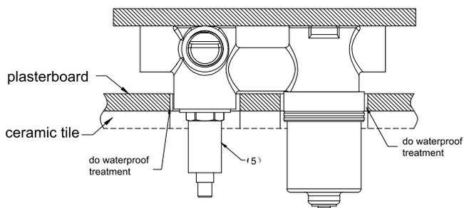
7. Install sleeve onto diverter, do waterproof treatment for gap of plasterboard and body.
