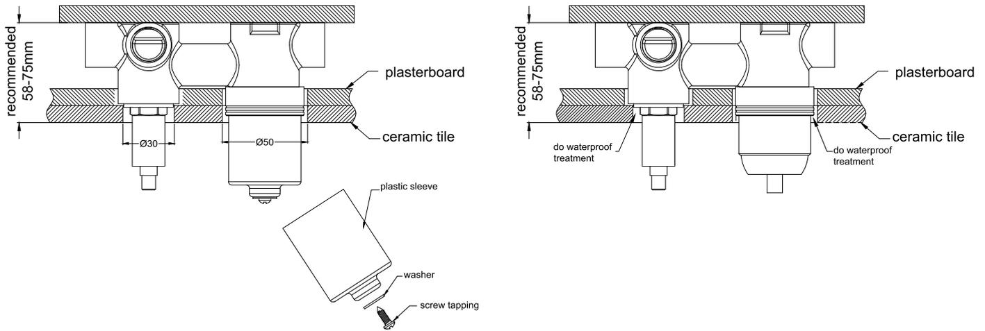
1. Install ceramic tile after drilling a  $\phi 50$  and a  $\phi 30$  hole according to above picture.
