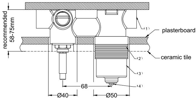
1. Fix body (1) on noggin and ensure installation depth is 51-68mm from noggin to ceramic tile. Caution: Do not take off plastic sleeve on body.
