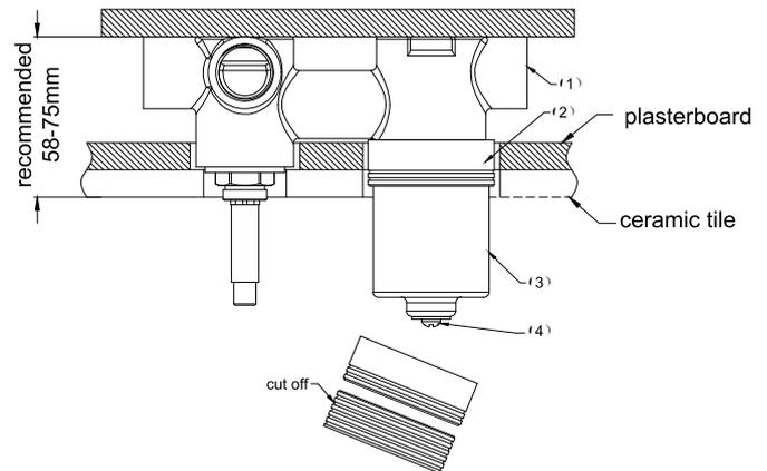
4. When the installation depth is 58-70mm, make a mark on plastic sleeve (2) at 2-4cm from ceramic tile surface to body. when the installation depth is 71-75mm, make a mark on plastic sleeve (2) at 4-7cm from ceramic tile surface to body.
