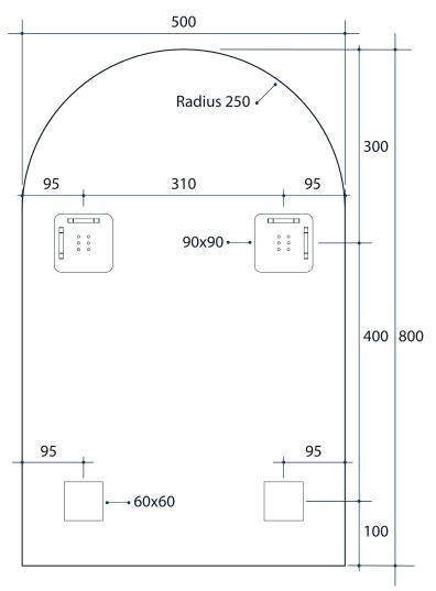
Note: All dimensions are in millimetres (mm)
