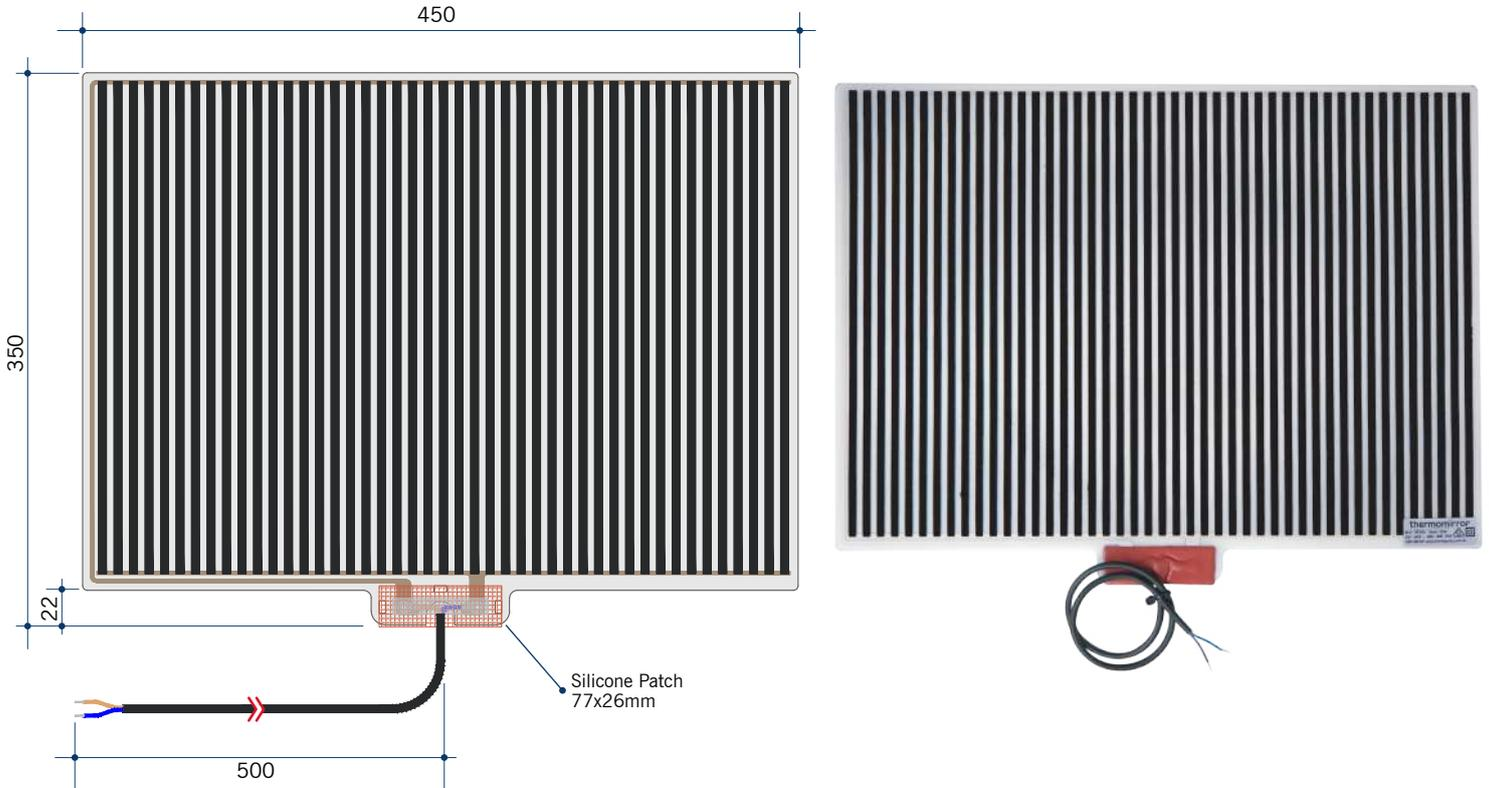
Note: All dimensions are in millimetres (mm)
