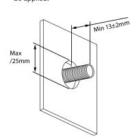
**2.** Apply thread tape (or similar) to the ½" connection, then screw the rail connector to the connection.
