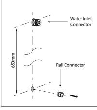
4. Check the grub screws are wound tight. Push the rail brackets onto the top and bottom rail connectors until they are against wall. Secure with grub screws.
