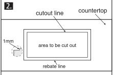
Use an appropriate cutting tool for your countertop material and cut along the template line.
