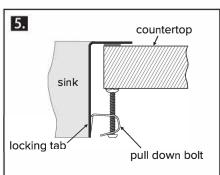
Fit the pull down bolts to the locking tabs. Tighten the sink to the countertop using a screwdriver.
