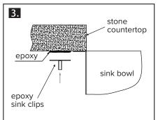
Ensure the underside of the sink is clean and dry.
