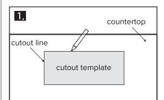
Place the cut-out template into the desired location and trace around the border of the template. Make sure the countertop is level, as this can affect the draining of water.
