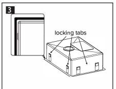
Ensure the underside of the sink is clean and dry. Test fit the sink to confirm the cut out is correct. Apply a bead of neutral cure silicone sealant (not provided) to the underside of the edge.
