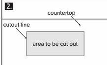
Use an appropriate cutting tool for your countertop material and cut along the template line.
