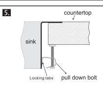
Fit the pull down bolts to the locking tabs. Tighten the sink to the countertop using a screwdriver.
