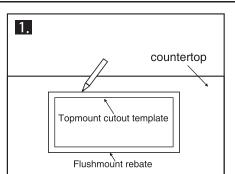
Place the cut-out template into the desired location and trace around the border of the template. Make sure the countertop is level, as this can affect the draining of water.
