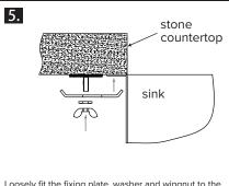
Loosely fit the fixing plate, washer and wingnut to the sink clip. Rotate the fixing plate so it secures the sink edge. Tighten the wingnuts; opposite corners first, and then any remaining nuts.
