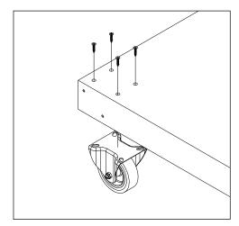
Use M6 Bolt and Nuts to assemble legs
