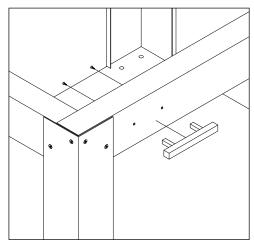
Use M5 Bolt and Nuts to assemble handle
