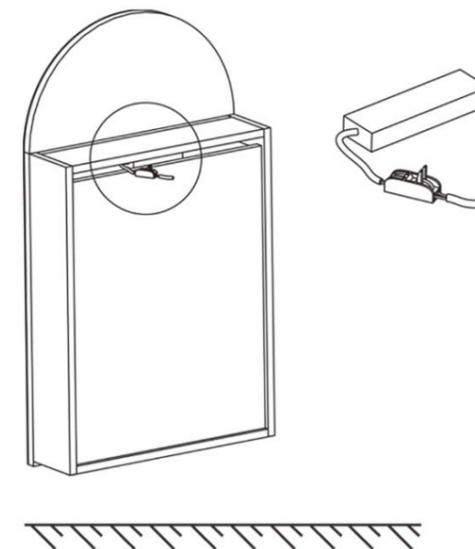
Connect power: Connect the 3-pin connector to the power line reserved on the wall, and then close the 3-pin connector. (LED Shaving Cabinet Only)
