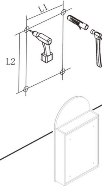
Drill the pilot holes into the pencil marks you made on the wall, punching the expanding rubber particles into the holes.
