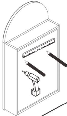
Level the shaving cabinet, and mark the holes on the back panel. Drill the holes.
