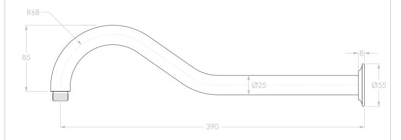
WORKING PRESSURE: 350 – 500KPA (INCLUDING COLD AND HOT WATER PRESSURE)
