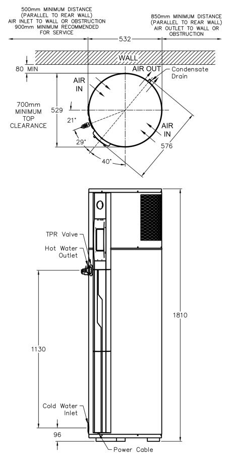
**Model 551180** There is a minimum clearance of 80 mm from a wall behind the water heater
