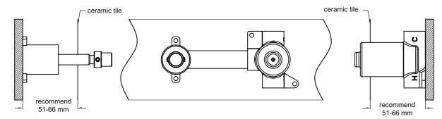
1. Fix body on nogging and ensure installation depth is 51-66mm from nogging to ceramic tile.
