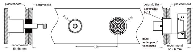
2. Put cartridge bell onto body and do waterproof treatment for the gap between cartridge bell and plasterboard and ceramic tile.
