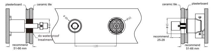
3. Adjust connecting rod and ensure depth is 25-28mm from the front of adaptor to ceramic tile.
