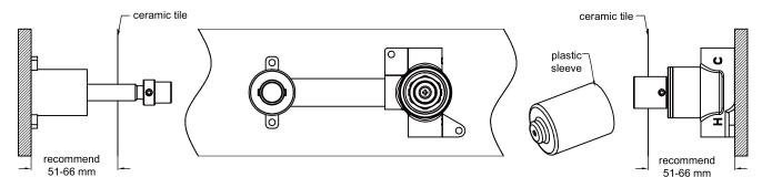
2. Connect cold water hose and hot water hose, take off plastic sleeve and conduct water pressure test for leak.
