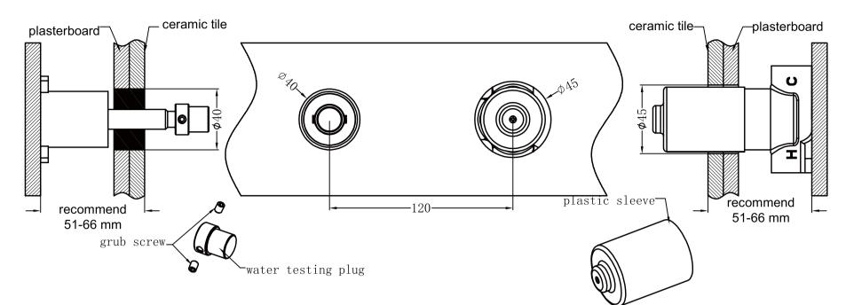
1. Remove plastic sleeve, grub screw and water testing plug.
