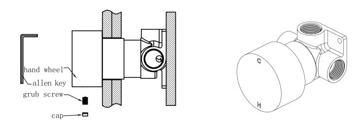
3. Make hand wheel into connecting rod, turn the hand wheel counterclockwise to the end. Then reinstall the hand wheel, make the "C" should be on twelve o'clock direction and "H" on the six o'clock direction, according to above picture. Then tighten grub screw of hand wheel by allen key, put cap into hand wheel.
