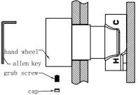
3.Put plate, washer and spout onto body successively, tighten grub screw of spout firmly by allen key.
