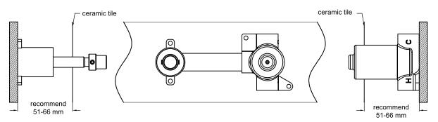
1. Fix body on nogging and ensure installation depth is 51-66mm from nogging to ceramic tile.
