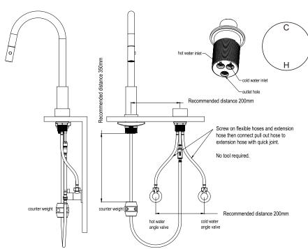
7. Turn the hand wheel counterclockwise to the end. Then reinstall the hand wheel, make the "C" should be on twelve o'clock direction and "H" on the six o'clock direction, according to above picture. Then tighten grub screw of hand wheel by allen key, put cap into hand wheel.
