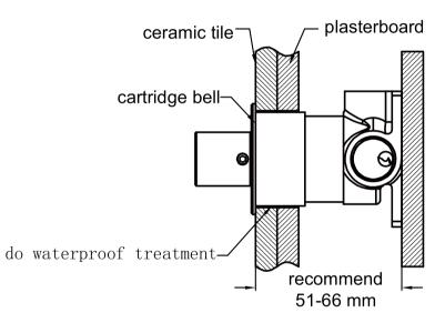
2.Put cartridge bell onto body and do waterproof treatment for the gap between cartridge bell and plasterboard and ceramic tile.
