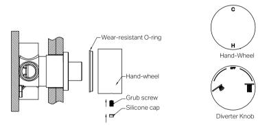
Follow step 10 to install the Hand-wheel and the Diverter Knoh
