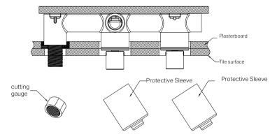
4. Remove the cutting gauge and protective sleeve.
