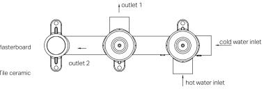
1.Fit off in-wall mixer body into wall structure, and ensure the installation depth is 51-66mm from the tile surface.
