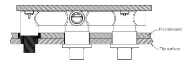
7.Apply waterproofing in the gap between the ceramic tile and the water outlet.
