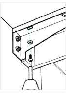
**2.** Fit the two mounting brackets to the bottom of the basin with the provided M5 x 10mm screws and flat washers and tighten. Please note the brackets are left and right specific.
