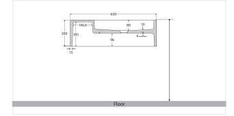
3. Hold the basin against the wall in the desired position according to the centre line and adjust to be flat and centred. Mark the position of the bracket fixing holes onto the wall. Remove the basin and drill four holes in the masonry wall using a 10mm masonry drill bit, to the required depth.
