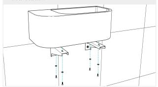
**4.** Place an anchor bolt into each drilled hole and remove the nuts and washers from the anchor bolts.
