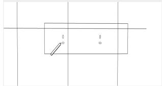
5. Place the basin in position against the wall, locating the anchor bolt threads through the holes in the basin brackets. Place the flat washer, a spring washer and nut onto each anchor bolt. Tighten the nut on each anchor bolt to secure the basin.
