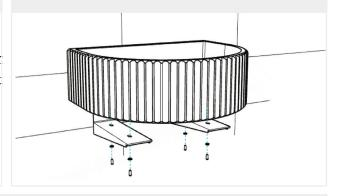
**7.** Install the tapware and the waste plug according to the installation instructions for the fittings. Connect the water supply pipe and the drainage pipe.
