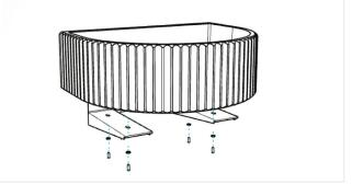
**3.** Measure and record the mounting hole locations of the basin mounting brackets. Transfer the mounting hole locations to the wall according to the centre line and adjust to be flat and centred. Drill the four marked holes in masonry wall using a masonry drill bit, to the required depth. Push the supplied wall plug into each hole.
