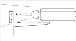
**6.** Screw the basin to the mounting brackets with the provided M5 x 10mm screws and flat washers and tighten.
