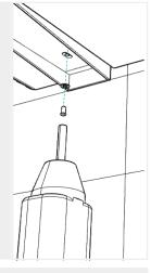
**5.** Place the mounting brackets in position against the wall, locating the wall plug holes through the holes in the basin brackets. Screw a mounting screw into each wall plug to secure the mounting brackets to the wall.
