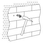
3. Insert the expansion plugs into the drilled holes using a hammer.
