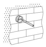
1. Use the mounting bracket to mark the drilling points on the wall.
