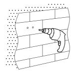
2. Use an electric drill with a 6mm drill bit to drill holes at the marked points.
