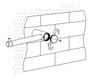
6. Install the rod of the toilet roll holder by tightening the grub screw, and screw on the cap.
