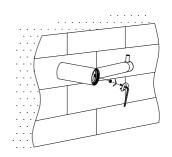
4. Remove the rod of the toilet roll holder by unscrewing the grub screw.
