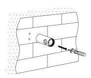
5. Position the rod bracket hole to the left and secure the bracket with expansion screws, as shown in the image.
