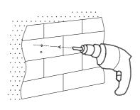
2. Position the fixing blocks at the marked spots. Mark the drilling points through the fixing block holes.
