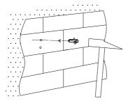
3. Use an electric drill with a 6mm drill bit to drill holes at the marked points.
