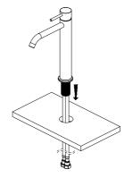
2. Place the mixer body and pass the Pex hoses through the hole in the counter-top. Ensuring the O-RING sits within the bottom groove of the base plate to prevent water leakage through the cabinet.
