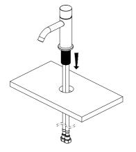
2. Place the mixer body and pass the Pex hoses through the hole in the counter-top. Ensuring the O-RING sits within the bottom groove of the base plate to prevent water leakage through the cabinet.
