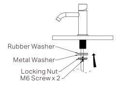
3. Install the rubber and metal washers, tighten the locking nut securely with the two M6 screws to ensure the mixer is firmly attached to the counter-top.
