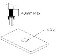
1. Pre-drill or create a hole with a diameter of 35mm at the proper location. Please note that the thickness of the surface should be between 3mm-40mm.
