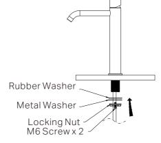
3. Install the rubber and metal washers, tighten the locking nut securely with the two M6 screws to ensure the mixer is firmly attached to the counter-top.
