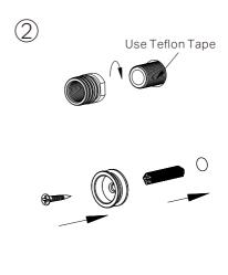
Check that G1/2 outlet thread is the correct length as shown.
