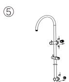
Insert the divertor and shower bracket into the water inlet and mounting bracket. Secure firmly with grub screws.
