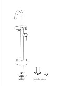
9. Push floor standing mixer into the base plate. Red water connector into H. Blue
