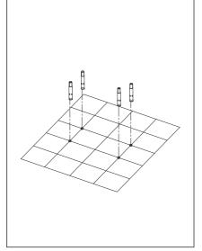
4. Discuss with your plumber/installer how the plumbing will be run, if elbows are needed we recommend installing to body now. Secure the base plate to the floor with supplied fixings.
