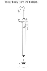
8. Add the base plate, adjust the hole direction to fit into the base plate.
