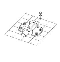
5. Connect hot and cold water according to the diagram, check whether there is leakage, and then lay cement and tile according to the diagram. Leave the 90 x 60 mm spare hole for installation.
