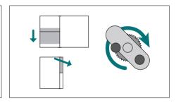
To adjust the drawer down (forward tilt) turn clockwise.
