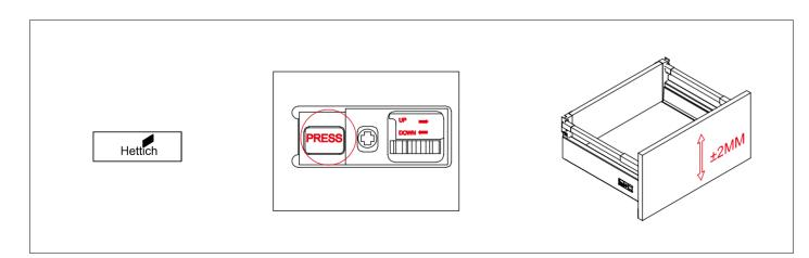
Remove the cap. Adjust the height of the drawer by rotating the knob.
