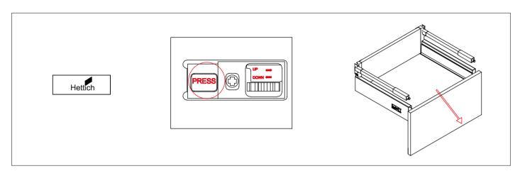
Remove the cap. Press the "PRESS" to split the drawer panel and font.
