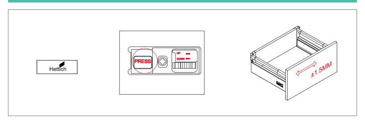
Remove the cap. Adjusting the nut to make the drawer panel left or right.
