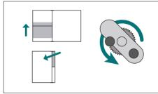
To adjust the drawer UP (backwards tilt) turn anticlockwise.
