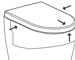
5. Push button and lift seat straight up to remove.
