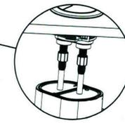
Button rods can be adjusted by screwing up or down
