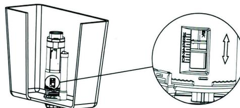
Full flush volume can be adjusted by changing the residual water level in the cistern.
