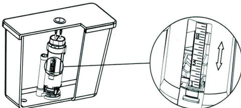
Half flush volume can be adjusted by moving the side float up or down.
