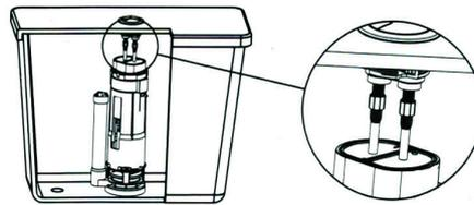
Button rods must be just clear of the valve pads
