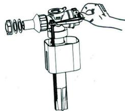
1. Unclip the float arm from the adjustment screw
