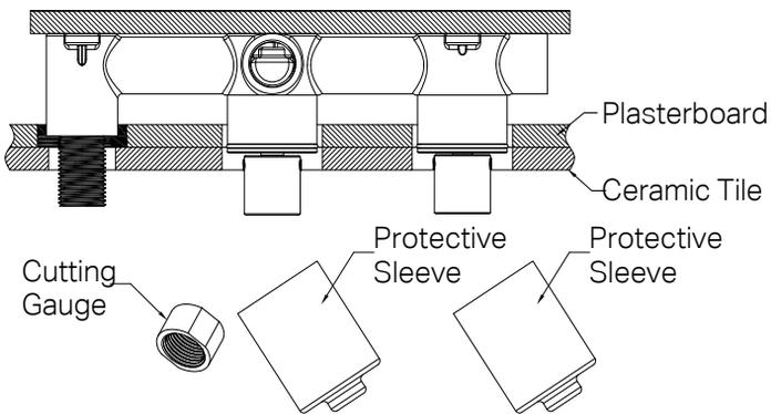
3. Trim any excess thread, and then remove the cutting gauge and protective sleeves.
