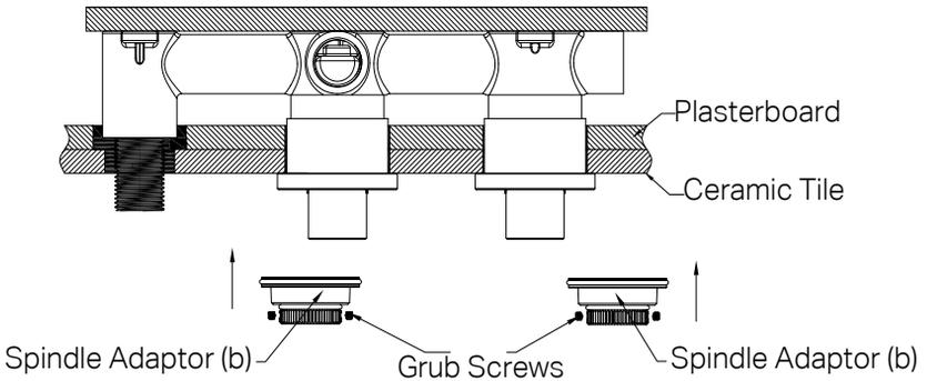
6. Use silicone sealant to seal the gap between the tile, wall plates and the G1/2 outlet.
