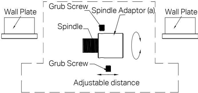
4. Adjust the two spindle adaptor (a) to the optimal length, ensuring a distance of 24-27 mm from the tile surface, as shown in the diagram.
