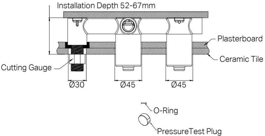
1. Drill two Ø45mm and a Ø30mm holes in the ceramic tile, then position it as shown in the above image.
