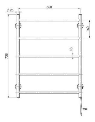
Electricity Input: 240V, 50Hz | Power Rating: 62W | IP Rating: IPX5 | Connection position: Bottom right | Connection type: Plug-in or Hardwire
