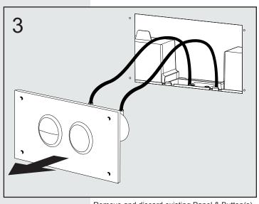
Remove and discard existing Panel & Button(s), leaving tube(s) connected to the cistern. Tubes installed in wall cavities should be left in position.
