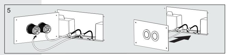
Using the Ø6mm pneumatic tube provided (cut to length as required), firmly make the connection(s) between both the rear of the button(s) and the smaller end of the "Cistern Bleed" adaptor(s).
