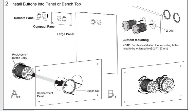
A. Insert threaded Button Body of your new button into your new Replacement Panel or Custom Mounting.
