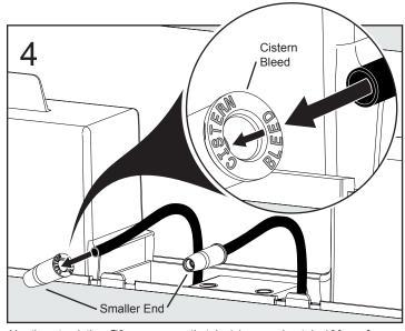
Neatly cut existing Ø8mm pneumatic tube(s) approximately 100mm from the cistern connection point.
