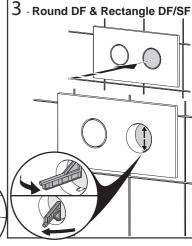
Depress the full flush button and use the Allen Key to lock the Face Plate to the Mounting Panel top & bottom.
