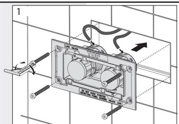
Remove Face Plate from the assembly and set aside. Push the Pneumatic Tubes into the rear of the Mounting Panel assembly ensuring the correct tube is matched with the corrosponding button. Use the supplied Allen Key and Mounting Panel Screws to fix the assembly to the Tiling Box or Remote Mounting Box. (Note that the Tiling Box or Remote Mounting Box should be trimmed flush to the wall prior to assembly of the buttons.)
