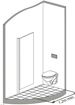
**16.** Ensure area 1.2m directly in front of panel is clear for calibration. Calibration is complete when the panel stops flashing. Flush panel to calibrate servos.
