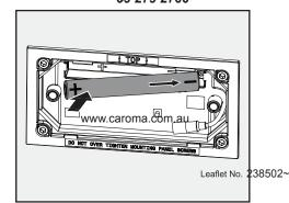
**11.** Install battery noting negative to right side of panel.
