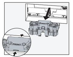
**4.** Squeeze clips at front and rear of bellows bridge and lift up and out of the cistern.
