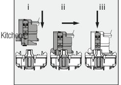
**7.** Install Actuator Bridge into position. Push down blue side sliders to lock.
