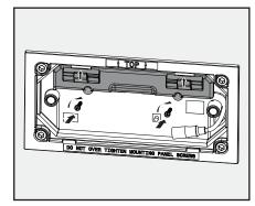
**12.** Engage Battery Cover clips under top edge and secure with provided screws. NOTE: Do not overtighten screws.
