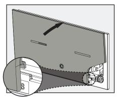
**14.** Engage bottom clips and rotate top of panel back flush against wall.
