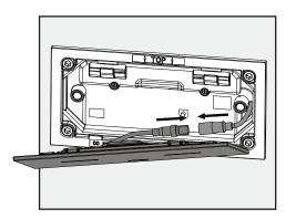
**13.** Securely connect Button Panel cables to Button Backing Assembly. NOTE: Once cable is connected you have 20 seconds before calibration comences.
