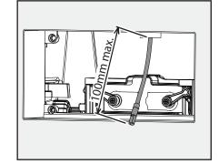
**8.** Ensure power cable and Actuator Bridge cable are accessible but don't extend beyond wallface by more than100 mm. Turn on power supply.
