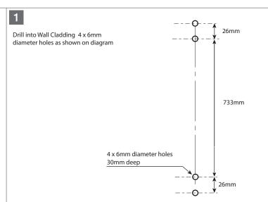
Push 4 x Plastic plugs into drilled holes. Place Rail Assembly over drilled holes . Fit screws provided. Tighten firmly.
